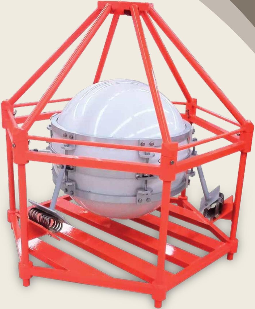
The INO sea-floor gravity meter uses the well proven CG-5 Autograv™ fused quartz sensor with electrostatic nulling which is incorporated into a submersible system. The INO uses an advanced electronics system with user-friendly software to provide microGal repeatability on the sea floor. The INO is designed for a depth of 600 m (1970 ft) with an Aluminum pressure sphere.
